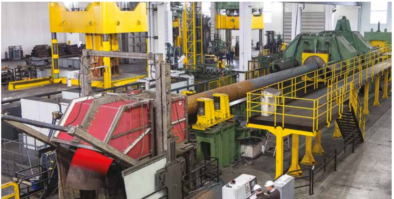
The large-dimension induction mandrel and bending machine MTC 1800 installed in the factory of Castel San Giovanni capable of unequalled production and a wide range of performances.
