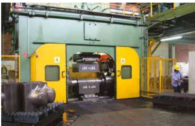
The cold forming machine in the Podenzano plant for the production of tees up to 16"
