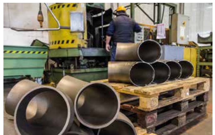
The cold bending machine in the Calendasco plant for the production of elbows up to 16"
