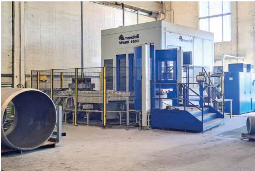
The Mandelli Spark1600 multitasking robot installed to optimize production
